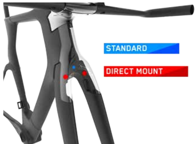
The different brake mount options are highlighted in red (Direct Mount) and blue (Caliper)
