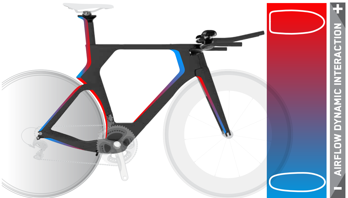
The F01-X230 parametric airfoil implemented on the Plasma 5
