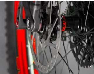
IDS-SL Dropouts Genius 700 Plus: Ready for Boost 148
