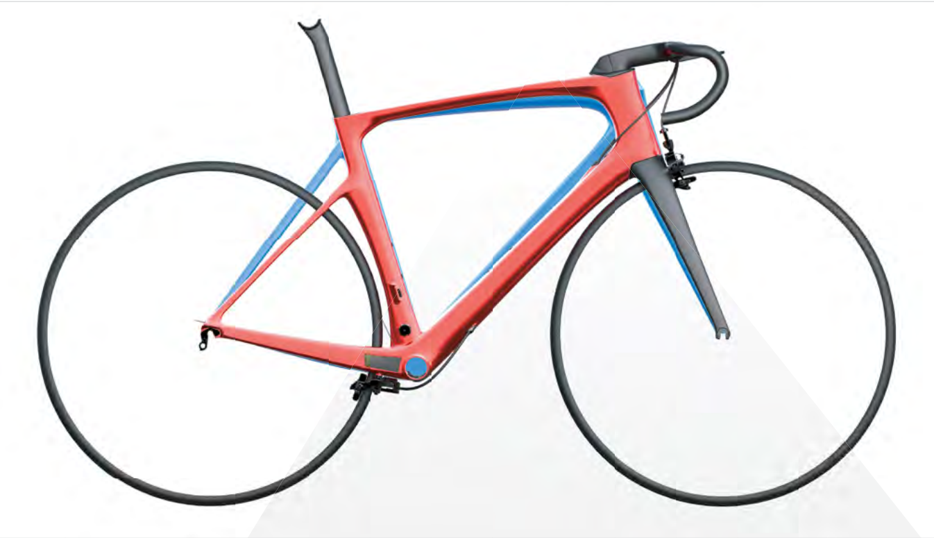
Superposition of the Foil 1 (blue) and Foil 2 (red): lowered seatstays and downtube avoid air stagnation.
